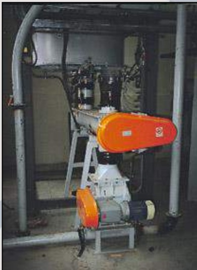
Coclea a truogolo (CT) Trough-shaped screw (CT)
