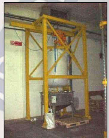
Scarico big bags. Discharge of big bags.
