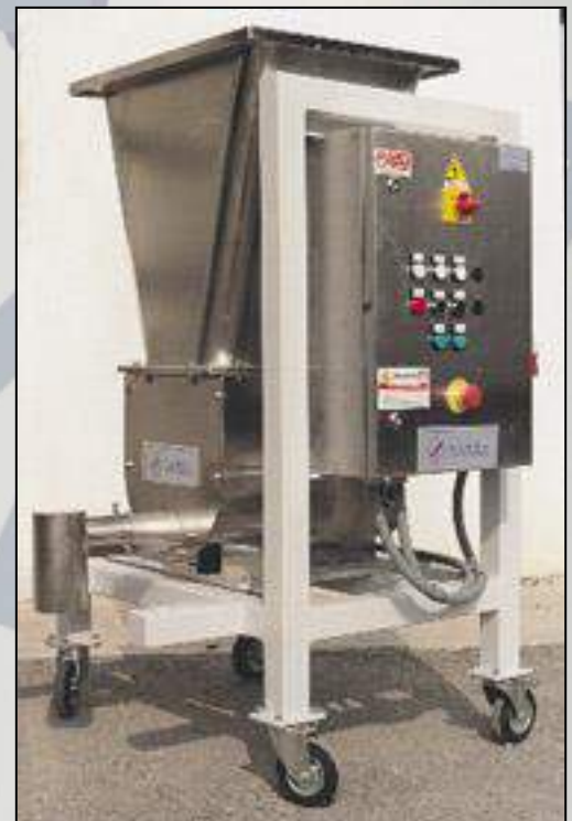
Microdosatore carrellato (MDC). Micro batchers
