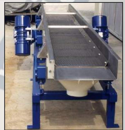
Canale vibrante (CV). Vibrating conveyor (VC).
