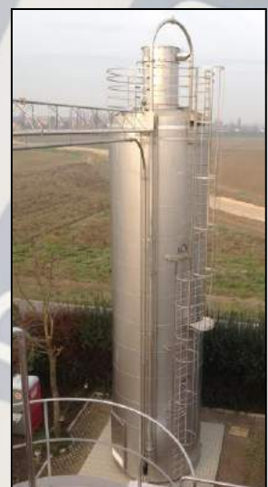
Silos in AISI304. Stainless steel storage bins.
